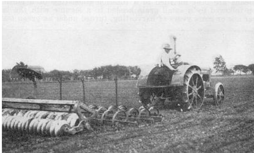
Fig. 2-Harrow and Cultipacker are Valuable Tools for Seed Bed Preparation.
