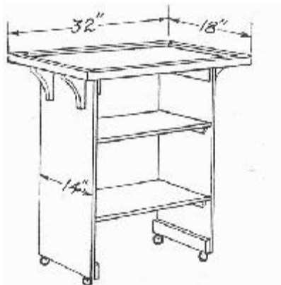
Fig. 8 illustrates a very simple, home made wheel tray which is equipped with common casters. A caster having a 3 inch wheel with rubber tire is preferable.
