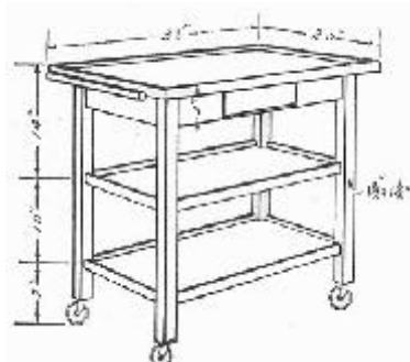
Fig. 9. The kitchen wagon shown in Fig. 9 is more carefully and substantially built, making a permanent piece of furniture. In building a kitchen wagon care should be taken to make the wheels far enough apart to insure stability, but not so wide as to prevent easy passage through doors.
